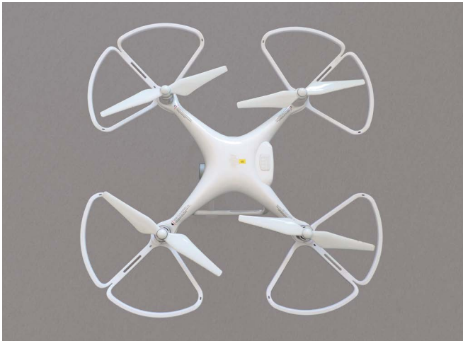
Abb. 8 Quadkopter in X- Bauform
